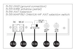
This three position slide switch allows selection of aerial input.
