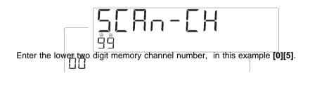
Now press the [.] key to inform the receiver that you are about to enter the higher memory channel number for programme memory scan. The channel legend "05" will be replaced by "--" when the [.] key has been pressed.
