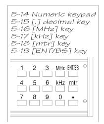
This key is also used as a separator when programming memory scan limits and memory delete limits.
