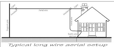
Magnetic balunderig wire aerials are betching very popular as they allow coaxial cable to be used as the down-lead from the wire aerial into the receiver. The balun transforms the impedance to a low level suitable for 50 OHM coaxial cable. In this instance the path of feeder is unimportant and chances of noise entering the aerial system reduced. The 50 OHM BNC aerial input of the AR3030 should be used and selected accordingly.
