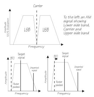
Above left: SSB true carrier re-insertion showing an unwanted signal in the passband.
